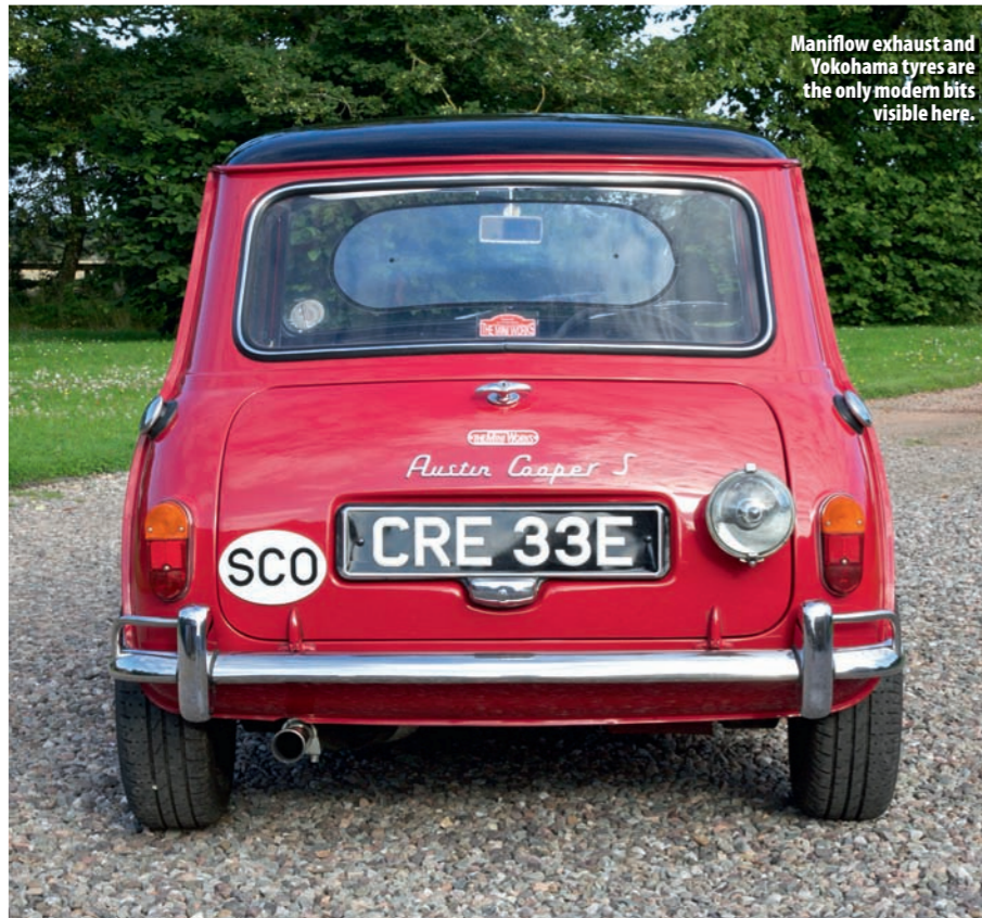
Oil cooler was standard on S from January 1966. Note careful exhaust installation preserving good ground clearance.
